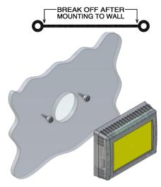
**Step 4:** Remove mounting tab before mounting on the wall.
