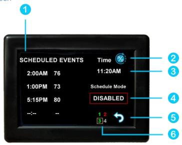
Set points may be changed on a time-based schedule. The mode used will be the heating or cooling mode set on the main screen.
